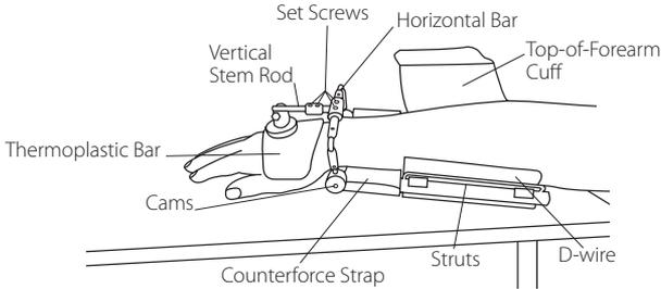
**STEP 3:** Align the struts with the midlines of the sides of the arm. See Figure 2.
