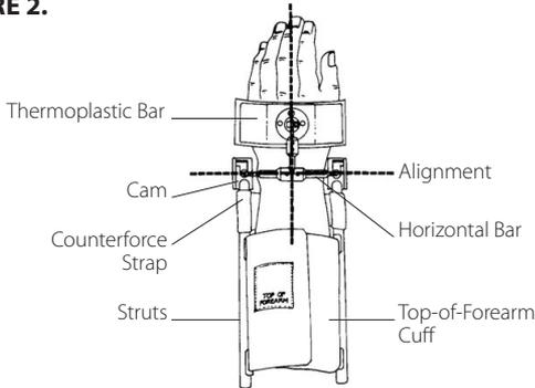
**STEP 4:** Align the cams with your wrist joint. See Figure 2.
