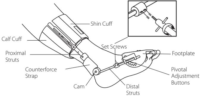
**STEP 2:** Slide the foot over the counterforce strap so that the top of the foot is centered below the footplate. See Figure 1.
